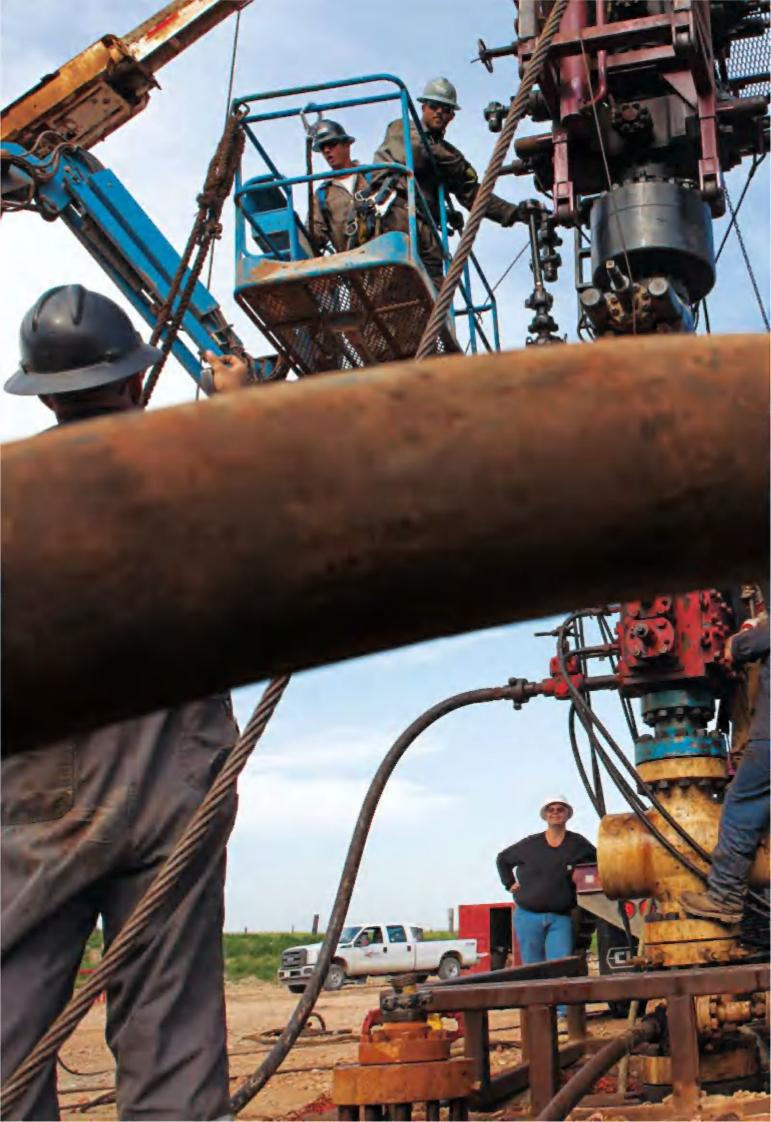
Near Epping, Arlin Fischer (hand on hip) oversees a workover rig, which allows the men to replace large drilling pipe with smaller, less expensive production pipe. Some 8,000 wells have been drilled in western North Dakota; there could eventually be 50,000.
